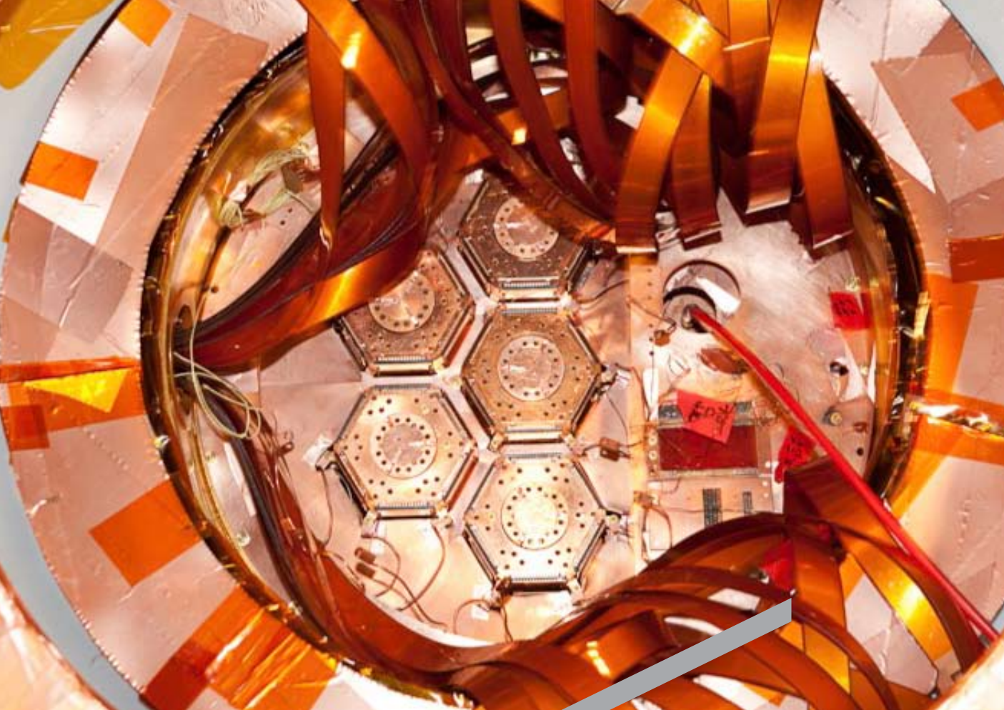
(Above) The tops of the detector towers in Soudan. Each tube carries six germanium and silicon crystals.
